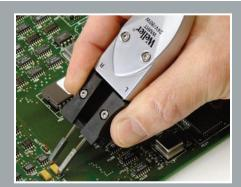
WMRT Desoldering Tweezers Quickly and easily desolders SMD chip packages as small as 0201.
